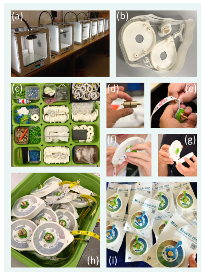
Figure 3. Photos of key steps in the manufacturing process. (a) Ultimaker 2 printers used to 3D print components of the mini-Secchi disk. (b) An example 3D print of the casing, bobbin and handle of the mini-Secchi disk. (c) Assembly of the components of the mini-Secchi disk after 3D printing the parts and printing the vinyl colour scale sticker, manufacturing the weight and the Secchi disk, and procuring the measuring tape. (d–g) Constructing the mini-Secchi disk. Having manufactured the weight (d), using either a metal lathe or a CNC machine, and bobbin (glued and finished), the weight is fitted into the bobbin and the measuring tape is stitched onto the bobbin (e). The bobbin is fitted into the casing (f) and measuring tape enclosed between the two sides of the casing (g) before being locked in place with the finger strap using the fittings. (h) The colour scale sticker is added before the handle of the device is fitted, lanyard added, and disk and weight attached to the measuring tape. (i) Examples of mini-Secchi disks produced for the REVIVAL project ( https://pml.ac.uk/Research/Projects/REVIVAL ).
