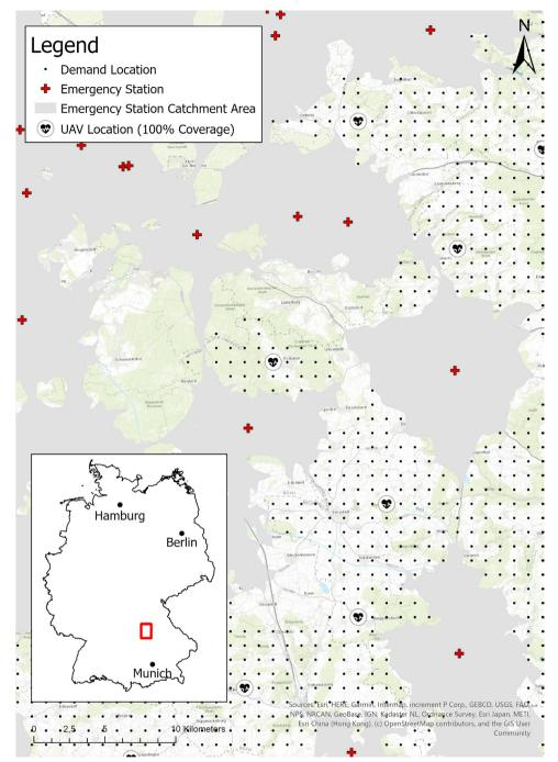
**Figure 1** Unmanned aerial vehicle (UAV) network configuration for universal coverage (100%) with adjoining emergency stations in an exemplary region in southern Germany.
