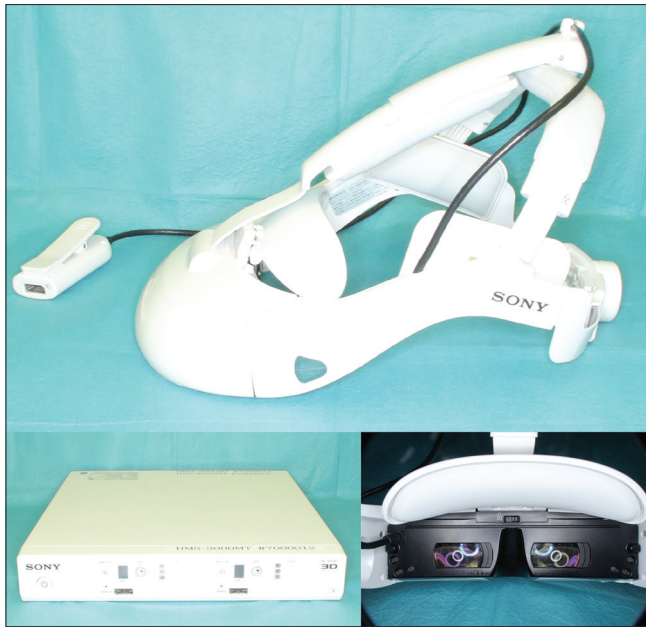
Figure 1: The head-mounted display system (HMM-3000MT; Sony Corporation, Tokyo, Japan). This equipment is a head-mounted display unit composed of a head-mounted image processor unit and a head-mounted display monitor, included a display
