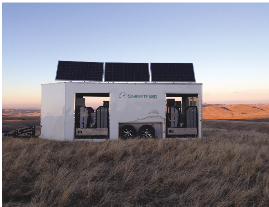
Figure 1. SmartFeed Pro (C-Lock Inc., Rapid City, SD USA) Feed Unit Trailer. Trailer has four feeding stations with two feeders randomly assigned to each treatment supplement.
