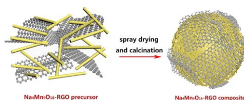
Figure 1. The schematic diagram of \text{Na}_4\text{Mn}_9\text{O}_{18} -RGO composite by spray drying.
