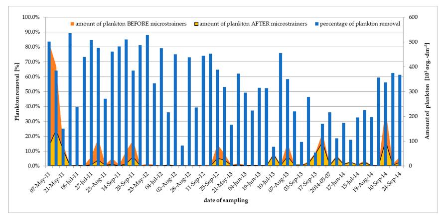
Figure 3. Efficiency of plankton removal after microstraining process in WTP Zawada from 2011 to 2014.
