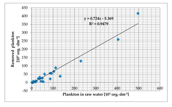
Figure 4. Relationship between amount of plankton in raw water and removed in WTP Zawada.
