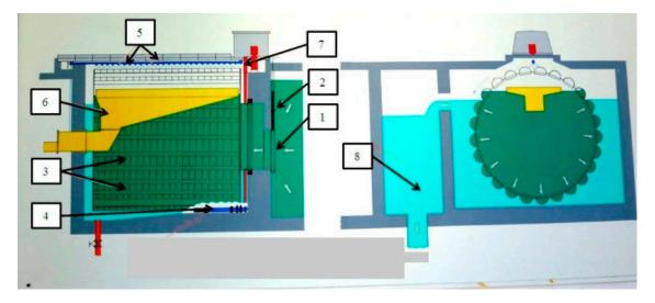
**Figure 2.** Microstrainers in WTP Zawada. **1** raw water supply; **2** slide flat; **3** mesh baskets; **4** submersible pump; **5** sprinklers; **6** drainage trough; **7** drum drive; **8** clean water outflow.
