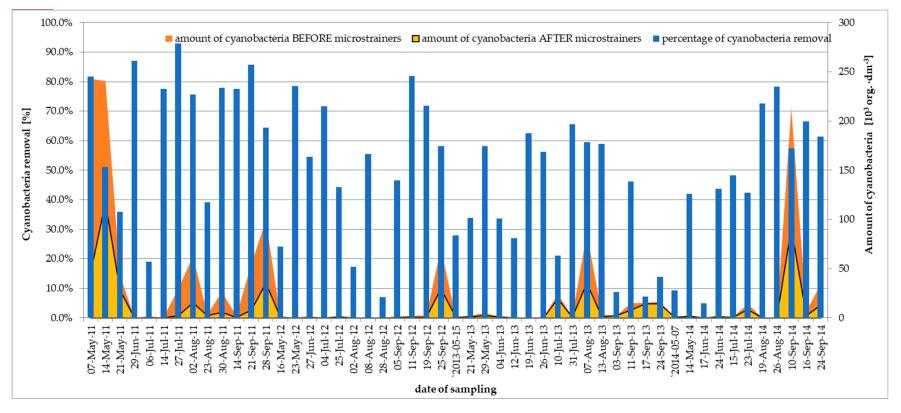
Figure 5. Efficiency of cyanobacteria removal after microstrainers process in WTP Zawada from 2011 to 2014.
