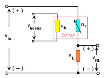
Figure 9. Setup experiment for measuring sensor response.
