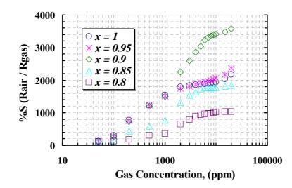
**Figure 15.** Response of samples to 0.01%, 0.02%, 0.05%, 0.1%, 0.2%, and 0.5% C<sub>4</sub>H<sub>10</sub>, measured at operating temperatures of 395 °C (x = 1), 385 °C (x = 0.95), 370 °C (x = 0.9), 430 °C (x = 0.85), and 440 °C (x = 0.80).
