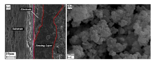
Figure 7. SEM micrographs: (a) cross-section of sensor layer, (b) surface of sensing film.
