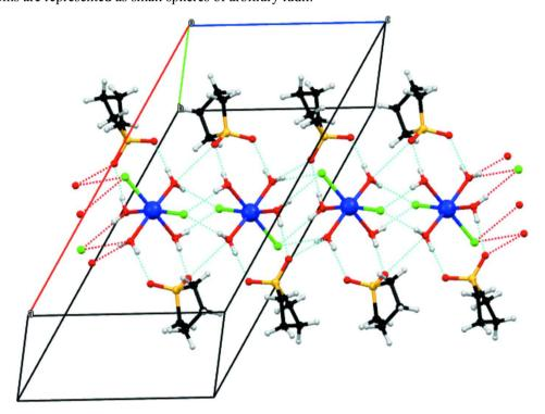
**Figure 2** Packing diagram of (I) showing the infinite chains of complex units and solvent molecule along the *c* axis.
