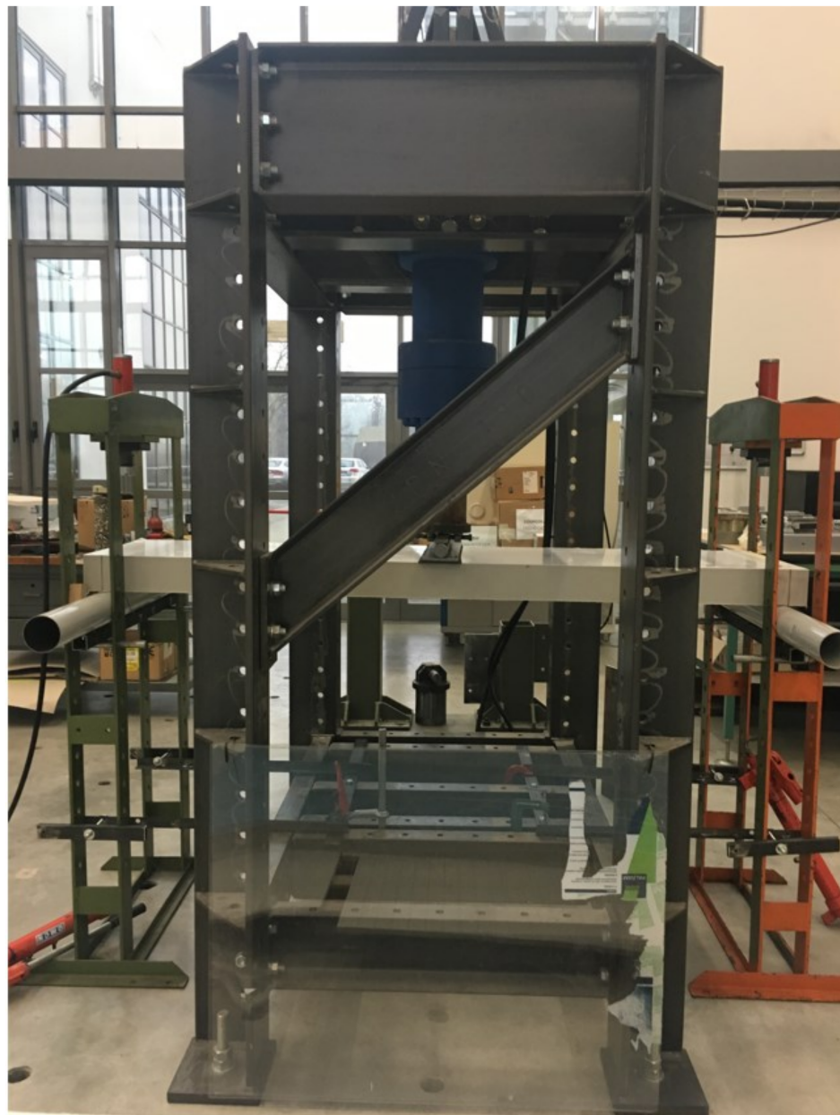
Figure 3. Electronically controlled hydraulic machine employed.
