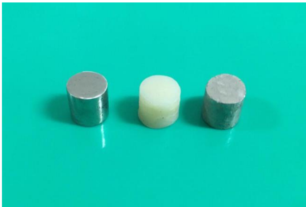
Figure 1. Backgrounds tested (from left to right: nickel–chromium, A2 shade composite resin, amalgam).
