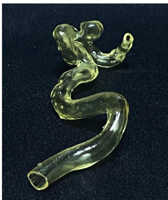
Figure 6. Hollow 3D printed model of ICA with an aneurysm on an ophthalmic artery.
