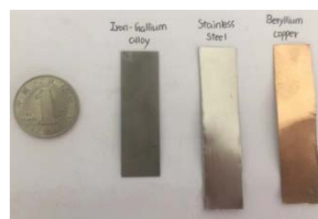
Figure 2. Photographs of active layer and elastic layer samples compared with a Chinese one yuan coin.
