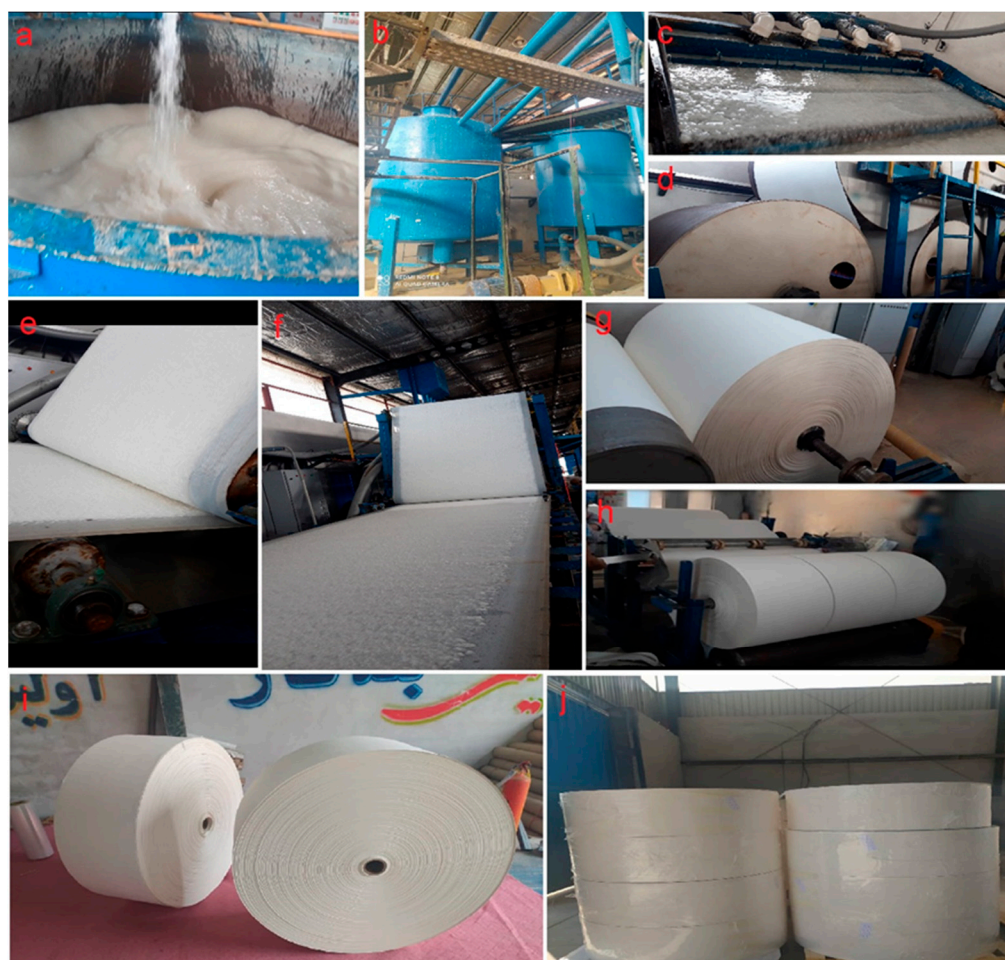
Figure 10. The processing of fluff pulp manufacturing. Pulper (a), storage towers (b), headbox (c), dryers (d), top and bottom wires (e,f), mother roll in the paper machine (g), three rolls in rewind machine (h) and packed rolls (i,j).
