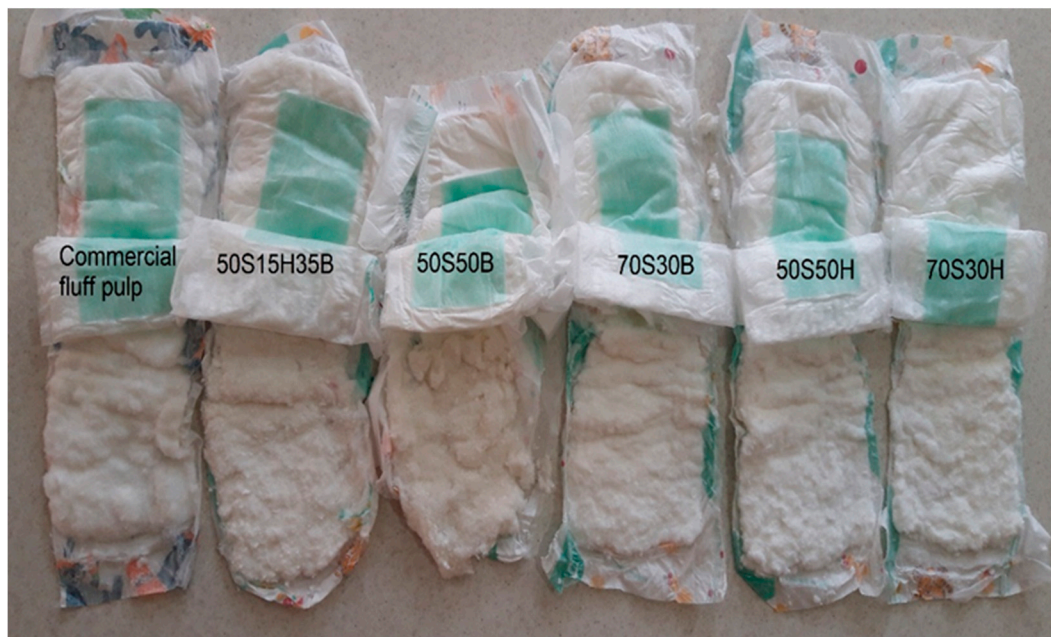
Figure 6. Defibration type of fluff pulp in the baby diapers.
