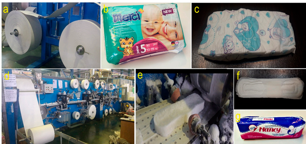
Figure 11. Different stages in production of baby diapers and sanitary napkins. Fluff pulp rolls working on the machine (a), baby diaper pack (b), baby diaper pad (c), BMT machine (d), fluff pulp in the shape of sanitary napkin (e), sanitary napkin pad (f), sanitary napkin pack (g).
