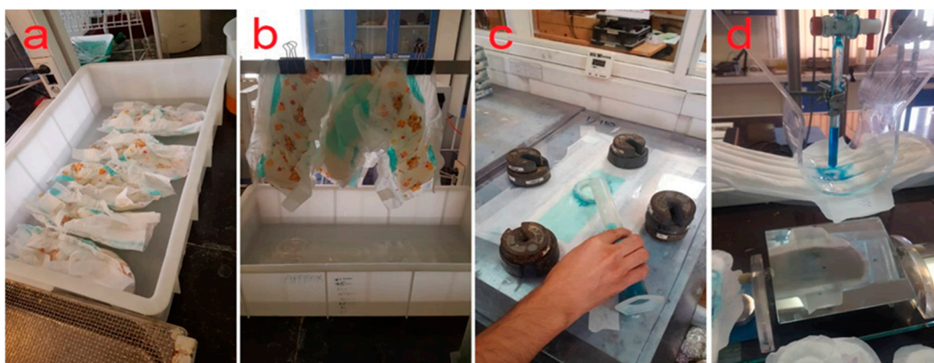
Figure 12. Experimental activity for testing of baby diapers and sanitary napkins. Absorption capacity test of baby diaper pad (a,b), rewet and absorption time of baby diaper pad (c), absorption capacity test of the sanitary napkin pad (d).
