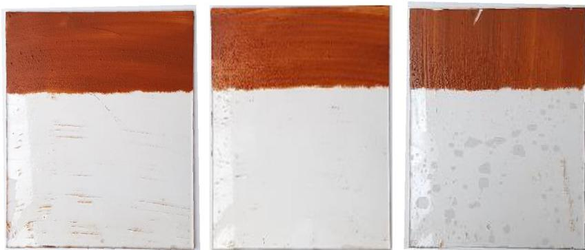
**Fig 10. The results of verification test performed under the optimal conditions.** Nozzle inlet pressure: 8 bar; spray distance: 0.2 m; injection angle: 40°. Image data results: 74.8% (average).
