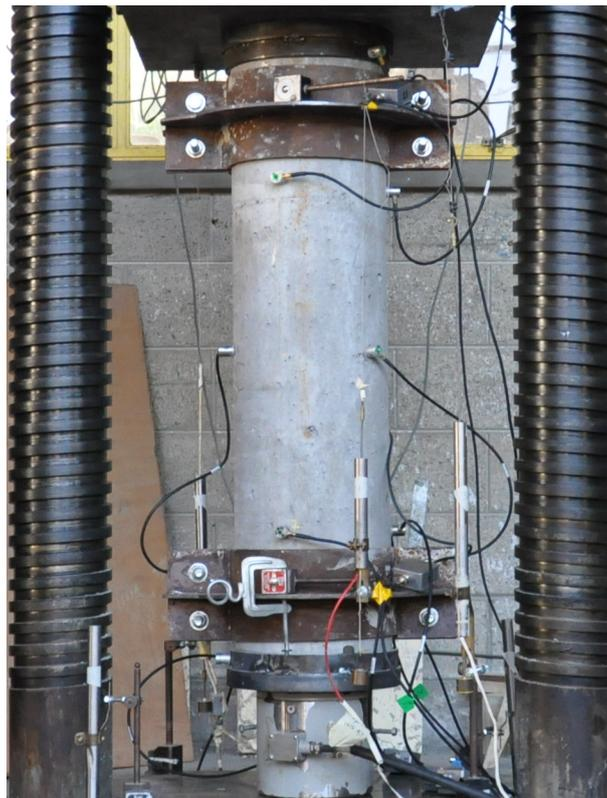
**Figure 2.** Test set-up of the reinforced concrete column specimens.
