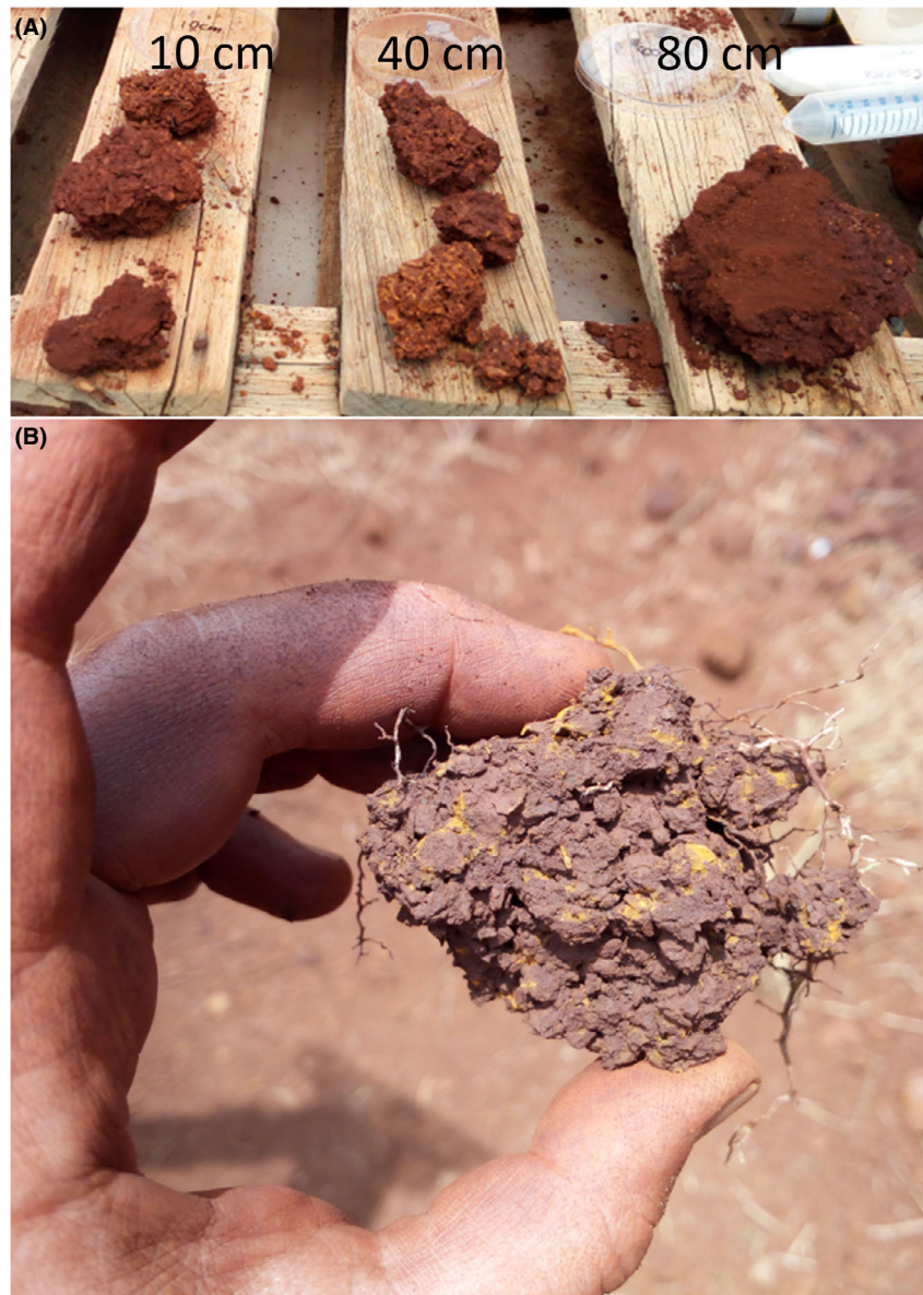
Fig. 3. Examples of re-cemented canga fragments recovered at end harvest from (A) the inoculated treatment (treatment D) at 10 cm, 40 cm, 80 cm; (B) the replicate of this treatment that was also seeded with canga plants (treatment E) at 40 cm depth.
