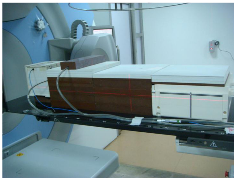
Figure 1 Solid water slab phantom used to measure peripheral doses. The positions of the 3 interest points are the breast, thyroid, and lens. The distance from the isocenter to the interest point is 35, 51, and 62 cm; the depth is 3, 2, and 1 cm, respectively.
