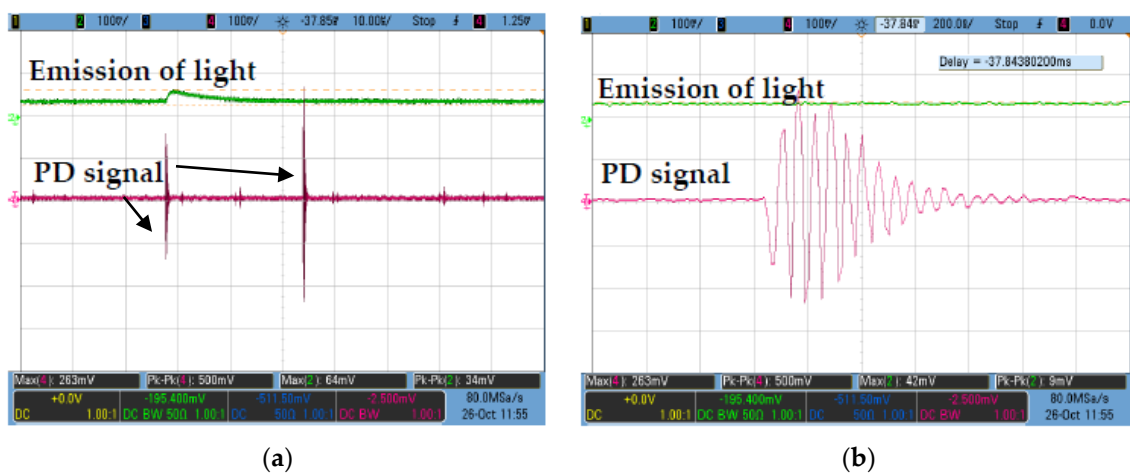
Figure 2. (a) Output voltage of the PD signal, (b) zoom in view for the output voltage of the PD signal waveform measured by impedance matching circuit (IMC).
