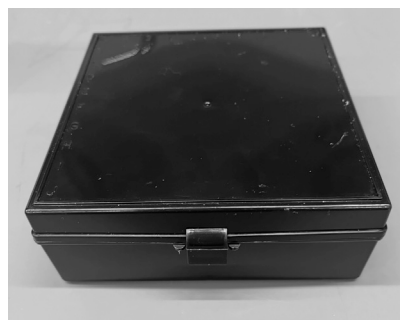
Figure 5. Light-proof box used for sample transfer
