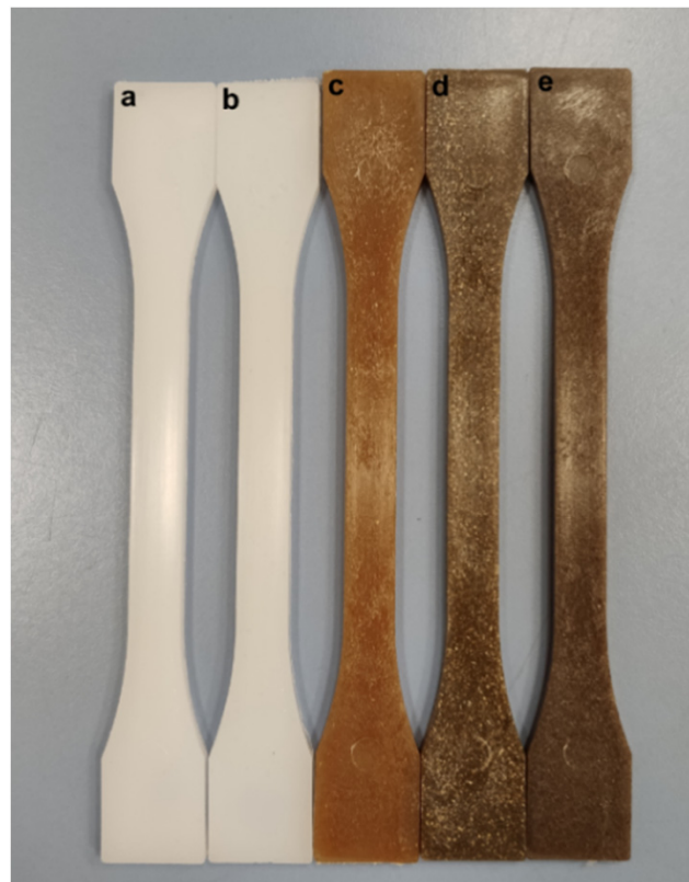
Figure 8. Visual appearance of the samples: (a) BioHDPE; (b) BioHDPE/PE-g-MA; (c) BioHDPE/Hemp/PE-g-MA; (d) BioHDPE/Flax/PE-g-MA; (e) BioHDPE/Jute/PE-g-MA.
