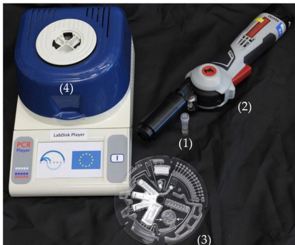
Figure 1. From [102], reused under CC-BY 4.0. (1) Tube contains the combination of the saliva sample, S. marinus control bacterium and steel beads. (2) Hand-held device (Terralyzer), where the tube is placed to carry out the mechanical lysis and homogenization of saliva. (3) The OralDisk, into which the lysate is pipetted in the chamber marked by the two white arrows. (4) The LabDisk Player instrument, which processes the OralDisk and performs real-time PCR. This system aims to integrate laboratory functions with a small chip, offering advantages like low sample volume, strong integration, and rapid response, as OralDisk delivers results in less than 3 h [115,116].
