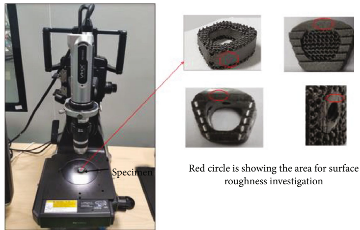
FIGURE 3: Set up for surface roughness measurement.
