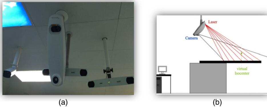
**FIGURE 1** (a) Sentinel, C-RAD laser, and camera, mounted in the ceiling in front of the gantry. (b) Sentinel, C-RAD scanner is connected to the personal computer (PC) running the c4D software
