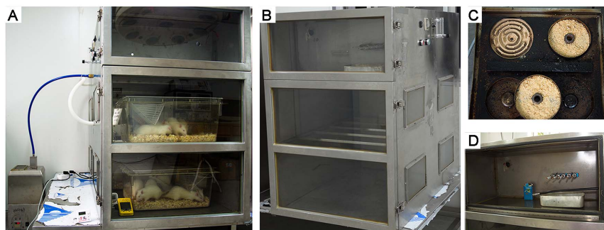
Figure 1. The whole-body smoke exposure apparatus. (A) The WS exposure apparatus primarily consisted of a wood burning stove, a piston pump and an inhalation chamber. (B) The CS exposure apparatus primarily consisted of a cigarette burning box, a piston pump and an inhalation chamber. (C) The wood burning stove had four independent heating wires (300 W), and the small iron trays were placed on the heating wire to smolder the wood sawdust. (D) The cigarette burning box had five cigarette holders. doi:10.1371/journal.pone.0096708.g001
