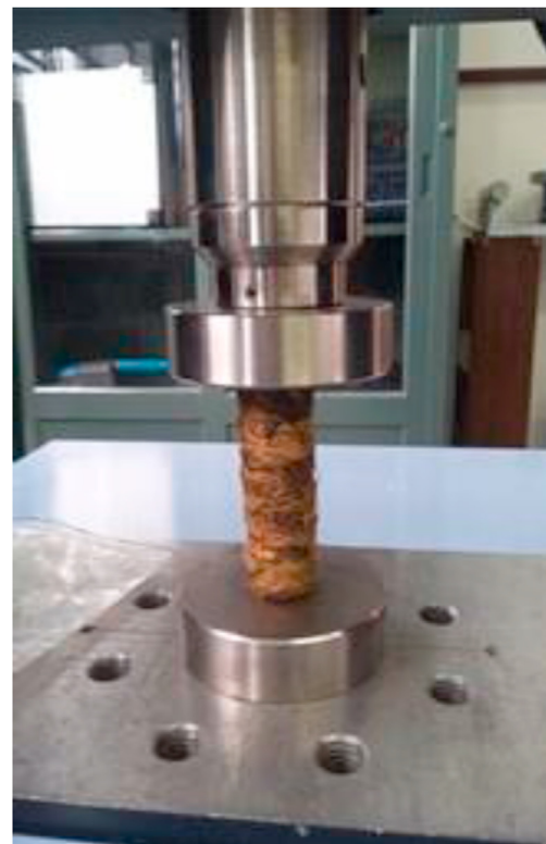
Figure 3. Experimental setup for compression testing of EFB briquettes. Source: Authors.
