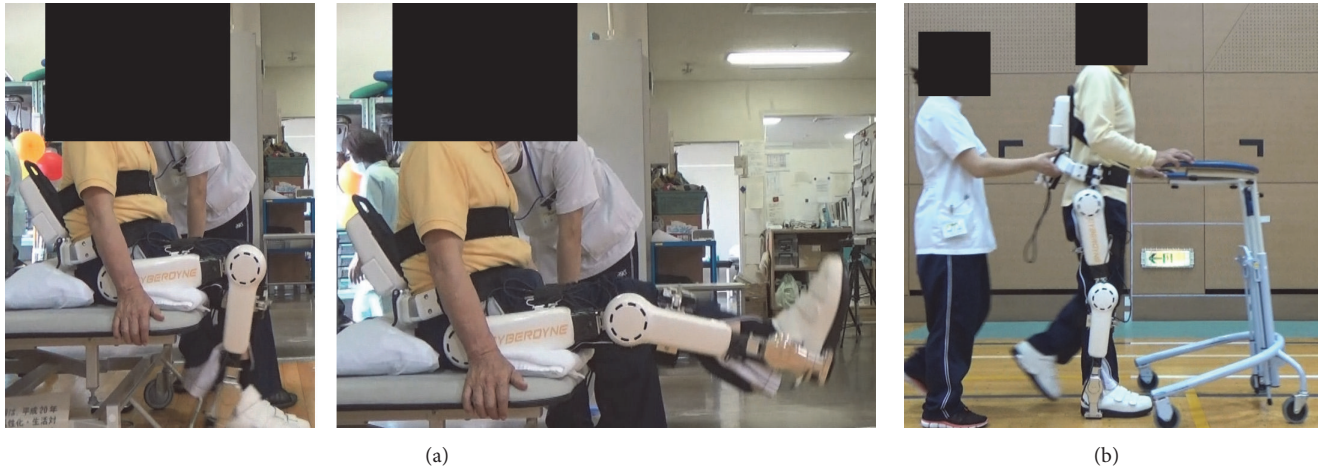
FIGURE 1: Photo of the hybrid assistive limb (HAL) on the patient (a). The patient is a 76-year-old male who underwent right TKA for grade 4 knee OA (Kellgren-Lawrence scale). Photo of the HAL training during walking (b).
