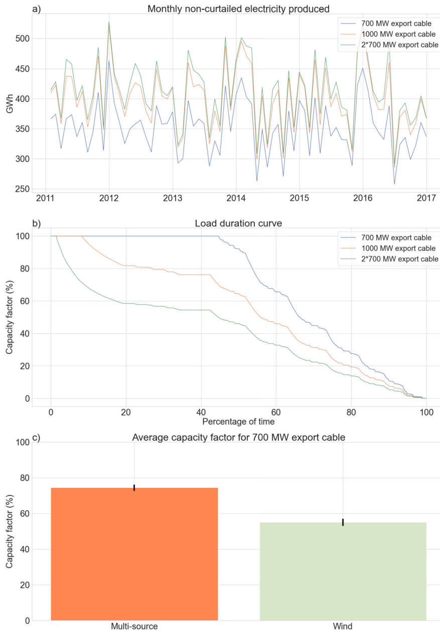
Fig. 3. a) Monthly non-curtailed electricity produced based on three different export cables 700 MW (blue), 1000 MW (orange), and 2 x 700 MW (green). b) Load duration curve for three different export cables: 700 MW (blue), 1000 MW (orange), and 2 x 700 MW (green). c) Average capacity factor for multi-source (orange) and wind (green) for a 700 MW export cable. The black error bars show the standard deviation of the timeseries.
