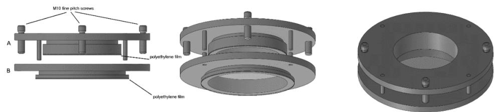
**Figure 2.** The figure shows a drawing of the device with the two membranes which seal the bottom of two containers A and B and the way it is assembled.
