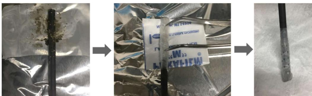
**Figure 1.** Sample preparation for cyclic voltammetric measurement: Step 1: Humins (HM) was distributed equally on a sheet of parafilm, and the graphite electrode was placed in the middle point of the sample area (about 2.5 cm of electrode's length); Step 2: The electrode was wrapped by that sheet of parafilm, and then  $\sim 20$  holes were perforated with tweezers to create at the sample area.
