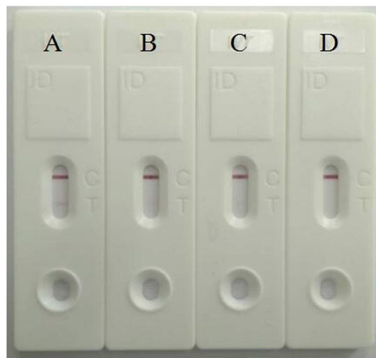
Figure 3. Mycoplasma pneumoniae detection. (B) Comparison the SWCNT/CGIC strip (A,C) with CGIC strip (B,D) without SWCNT. (A) and (B) 1 \times 10^3 copies/mL, (C) and (D) 1 \times 10^2 copies/mL.
