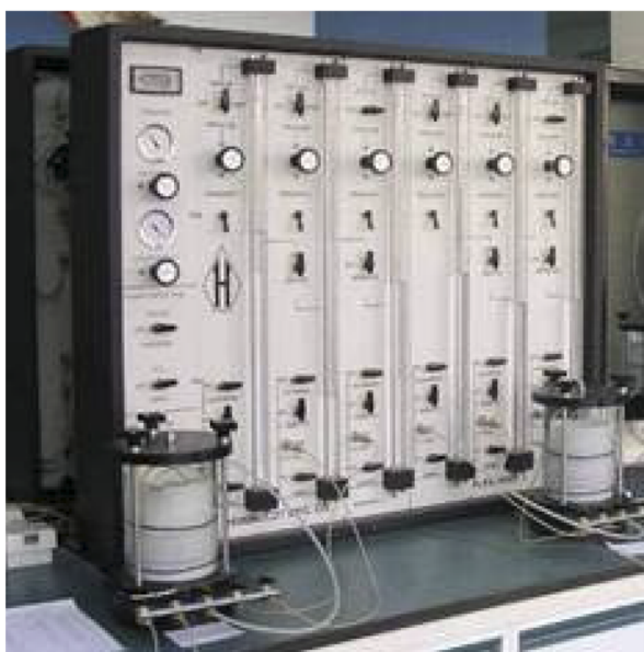
Figure 1. Schematic diagram of flexible-wall permeameter.
