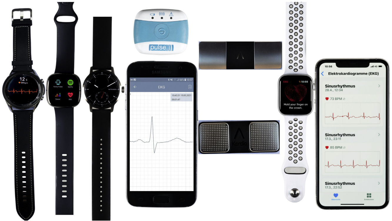
Figure 1 Wearable electrocardiographic (ECG) recorders. From left to right : ECG watches: Samsung Galaxy Watch 3, FitBit Sense, and Withings ScanWatch with a medical graded oximeter for SpO 2 measures. Right of the ScanWatch is the NextSENSE Pulse sensor 1-lead ECG recorder, which attaches to the chest by a belt or through electrodes. Displayed on the center smartphone is a wirelessly transmitted ECG signal, recorded with the Pulse sensor. Next are 2 different AliveCor Kardia devices: a 6-lead recorder—the KardiaMobile 6L ( top ), and a 1-lead recorder—the KardiaMobile ( bottom ). Right : Apple Watch with ECG recording capabilities displayed on a paired iPhone.
