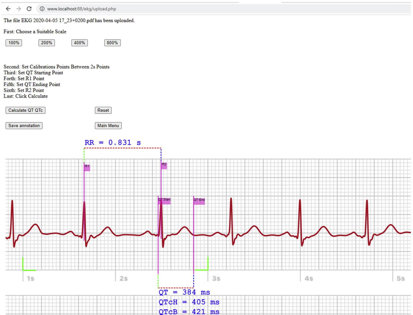
Figure 5 Self-made demonstrator application (APP) running in a Web browser for processing of uploaded electrocardiographic (ECG) PDF files. The APP is designed for physicians to measure the QT intervals of the ECG lead on the PDF and calculate the corrected QT interval. QTcB = Bazett formula; QTcH = Hodges formula.
