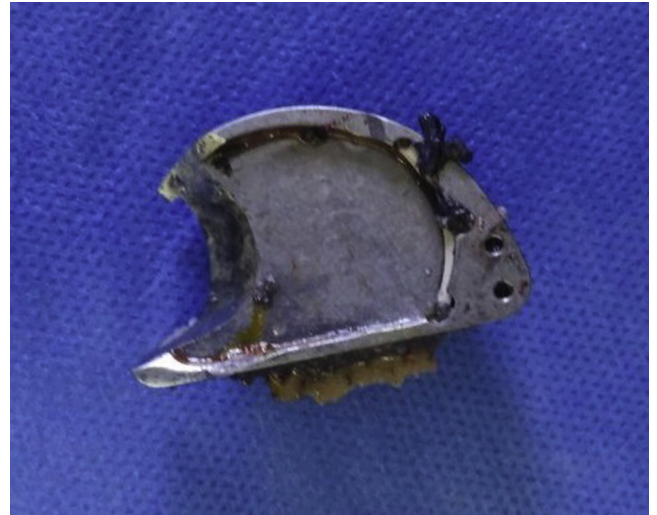
Figure 6. Metallic tibial component showing full thickness wear over the posterior one-third.
