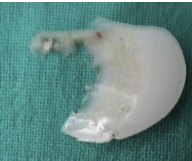
Figure 5. Polyethylene insert showing full thickness wear over the posterior half.
