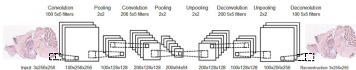
Figure 8. Illustration of convolutional autoencoder; the CAE consists of two convolutional layers and their two corresponding deconvolutional layers, and two max-pooling layers and their corresponding unpooling layers.
