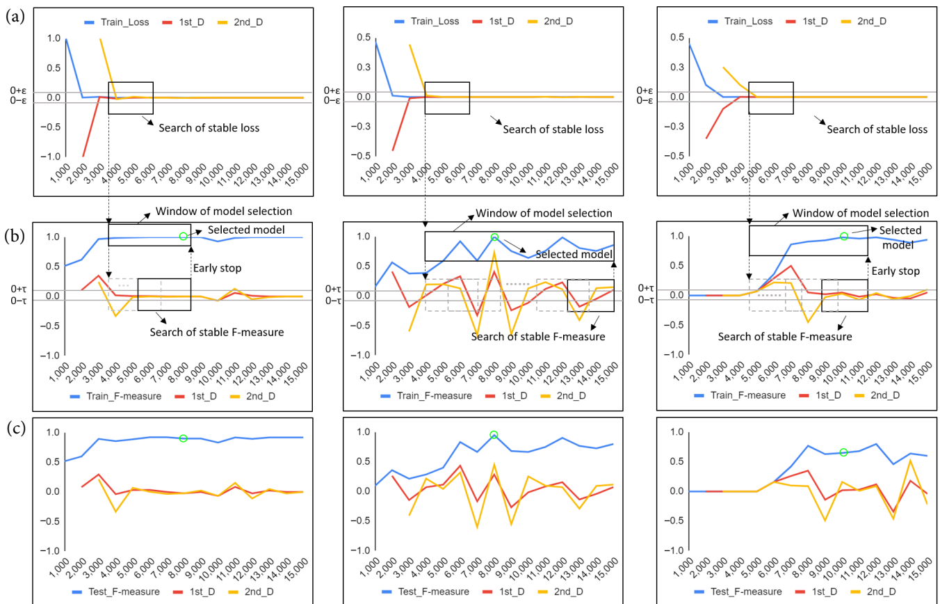
Figure 4. Illustration of the proposed model selection method with three examples: (a) loss values of models through iterations during training; (b) F-measure scores of individual models with different iterations on the training set; (c) F-measure scores of individual models with different iterations on the testing set. The blue lines indicate the measurement values, and the red and yellow lines represent the associated first and second derivatives, respectively. During training, the proposed model selection method computes the loss values and F-measure scores of trained models on the training set and further calculates associated first and second derivatives. If a stable loss is found in (a) where the first and second derivatives of the training loss converge for a continuous period, the starting point of the stable loss window is used as the starting point in model selection searching.
