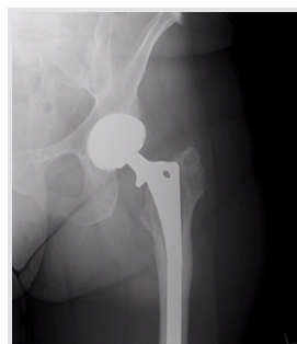
Figure 5: Radiographs demonstrating fracture of the left femoral stem.
