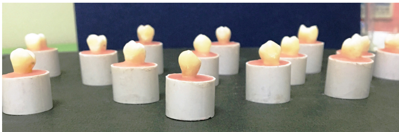
Figure 1 - Specimens mounted in self-curing acrylic resin.
