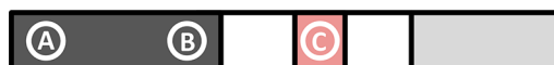
Figure 7. Lateral flow immunoassay highlighting the sample pad (A), the conjugation pad (B), and the test line (C).
