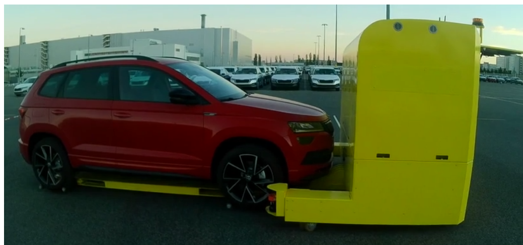
Figure 10. Autonomous vehicle prototype intended for car and heavy load transportation used for the vision-in-the-loop experiments. Courtesy of [44].
