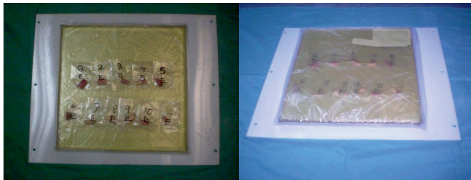
Figure 5 Cortical bone specimens placed in a board cover with a silicon pad layer before irradiation.
