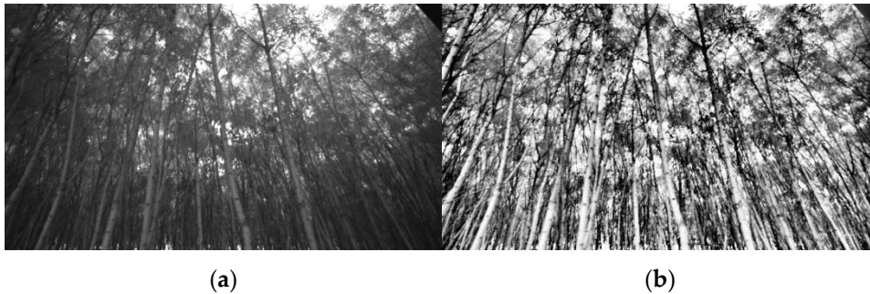
Figure 3. (a) Original grayscale image from the infrared imager; (b) grayscale image after applying the contrast-limited adaptive histogram equalization (CLAHE) algorithm.
