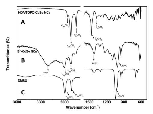
The narrow bands at 2956, 2917 and 2850  $\rm cm^{-1}$  can be ascribed to the  $\rm -CH_3$  asymmetric stretching and to the  $\rm -CH_2$  asymmetric and symmetric stretching, respectively, of the alkyl chains of TOPO and HDA molecules. At lower wavenumbers, the narrow bands at 1467 and 1378  $\rm cm^{-1}$  are ascribed to bending vibrations of C–H in the  $\rm -CH_2$  and  $\rm -CH_3$  moieties, respectively.
