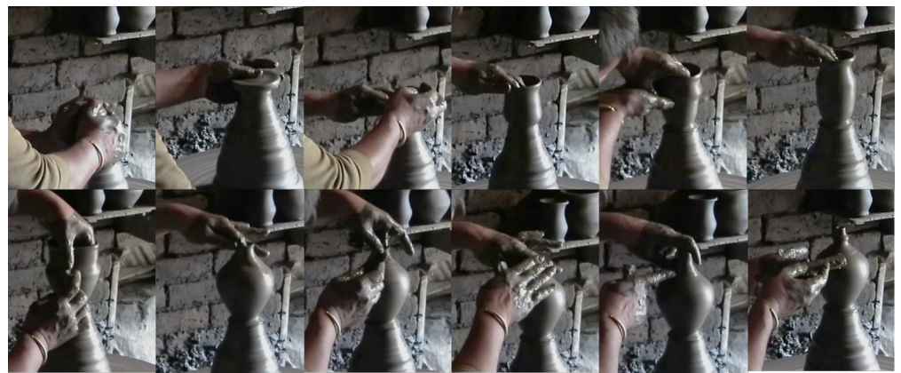
Fig 2. Examples of hand positions used during wheel-throwing. The images were extracted from a video recording of a Nepalese potter throwing a Money-Bank.
