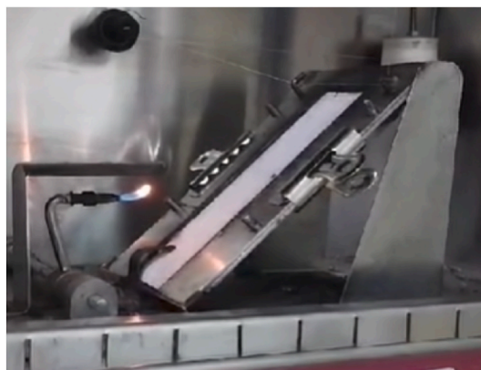
Fig. 2. 45° Angle flammability tester (testing lab).
