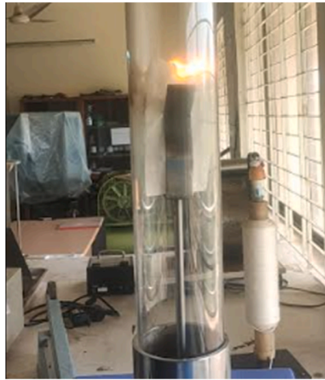
Fig. 3. LOI test of Type II solution treated sample, 63 % cotton, 35 % Polyester & 2 % Lycra woven fabric.
