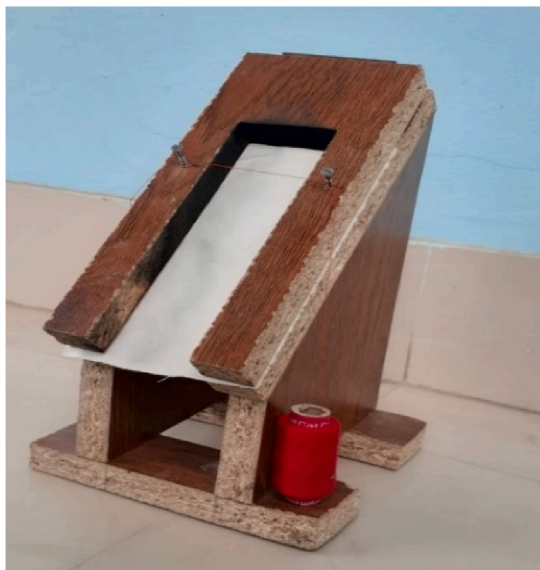
Fig. 1. 45° Angle flammability tester (manufactured by authors).
