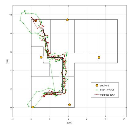
**Figure 16.** Tracking results obtained with Extended Kalman Filter (EKF) using Time Difference of Arrival (TDOA) values and proposed algorithm exploiting fusion of TDOA and gait parameters (modified EKF).
