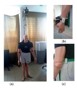
Figure 18. Manikin on the test site (a); and tags attached to the: wrist (b); and waist (c).
