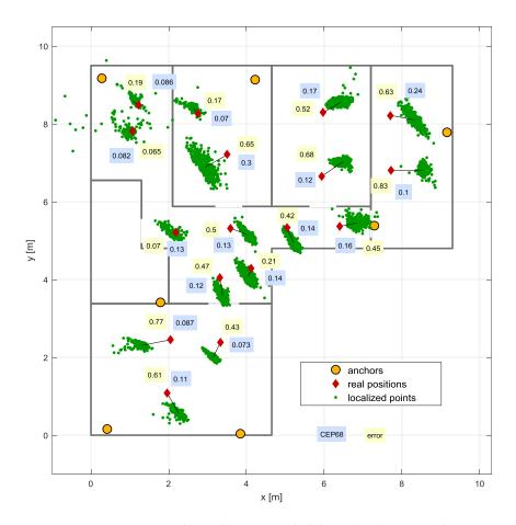
Figure 14. Positioning errors and Circular Error Probabilities (CEP) at particular test points.
