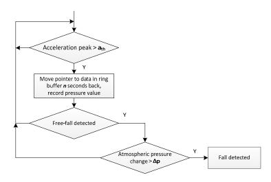
Figure 13. Fall detection algorithm.
