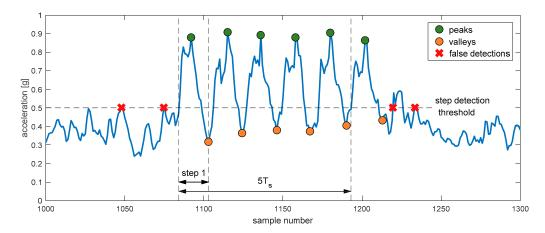
**Figure 9.** Acceleration measured for a sequence of six steps. Detected peaks and valleys are marked with green and red dots respectively. False step detections, which would occur for a simple threshold algorithm, are marked with red crosses.
