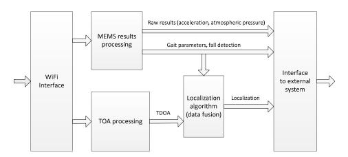
**Figure 7.** Data processing in the system controller.
