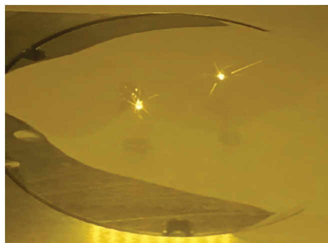
Fig. 3: 3D printing of the crowns using DMLS technology
