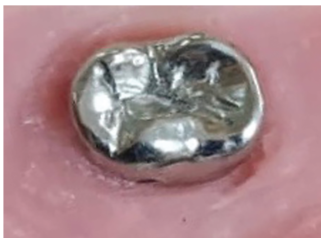
Fig. 5: 3D-printed metallic crowns using DMLS technology
