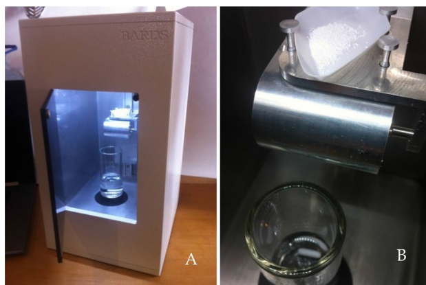
Figure 1. (A) External view of the BARDS instrument and (B) Tipper motor with a powder sample in a weighing boat ready for addition to the stirred solution below 27 .
