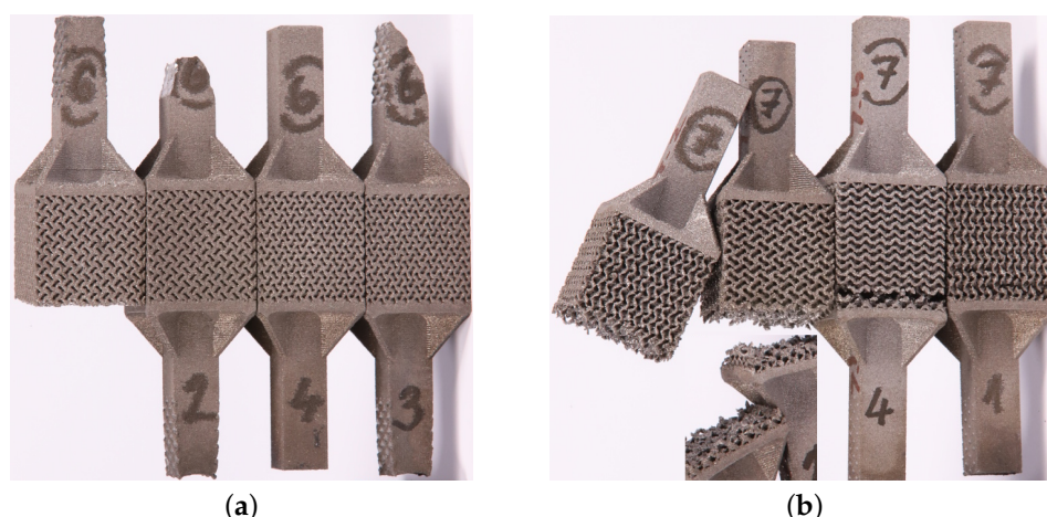
Figure 9. Fractured specimens undergoing tension: (a) failure at gripping section (samples 2, 3—porous structure corresponds to GII-2), (b) location of fracture surfaces near top base (porous structure corresponds to GII-3, specimens are positioned upside-down from the printing direction point of view).
