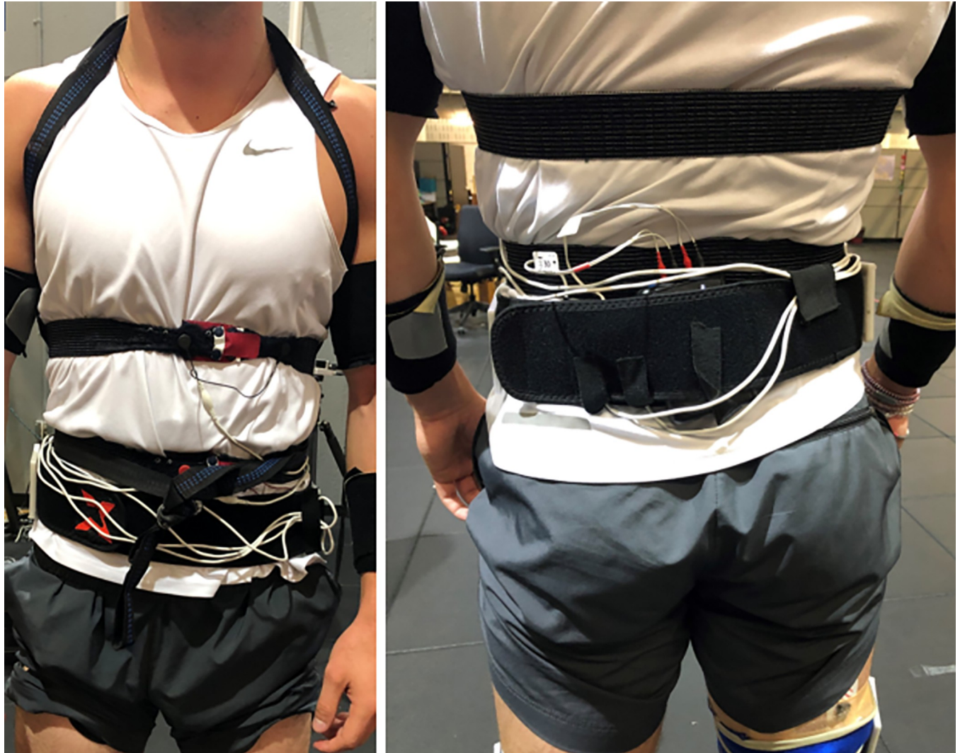
Fig 4. Equipment worn by participants. Anterior and posterior view of the equipment worn by participants while running. This equipment included two RIP belts, a heart rate monitor, a harness, and a neoprene belt. The neoprene belt housed the BioRadio, which was used to detect changes in voltage outputs of the belts, and additionally was where excess wiring from the RIP belts to the BioRadio was held down.
