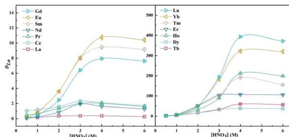
Fig. 3 Effect of  $\text{HNO}_3$  on the extraction of  $\text{Ln}(\text{III})$  by  $L^{II}$  in 40/60 (v/v)% *n*-octanol/kerosene (O : A = 1 : 1,  $[\text{Ln}^{3+}]_{\text{init}} = 3 \text{ mM}$ ).
