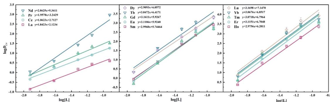
**Fig. 4** Dependency of  $\log D_{Ln}$  on extractant concentration in 40/60 (v/v)% *n*-octanol/kerosene (O : A = 1 : 1),  $[Ln^{3+}]_{init} = 3$  mM,  $[L^{II}] = 0.012$ – $0.12$  M.
