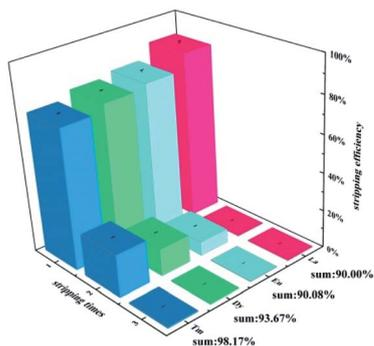
Fig. 6 Effect of the times of stripping on the stripping efficiency of La(III), Eu(III), Dy(III), and Tm(III) by nitric acid, O : A = 1 : 1, [HNO<sub>3</sub>] = 0.001 M.
